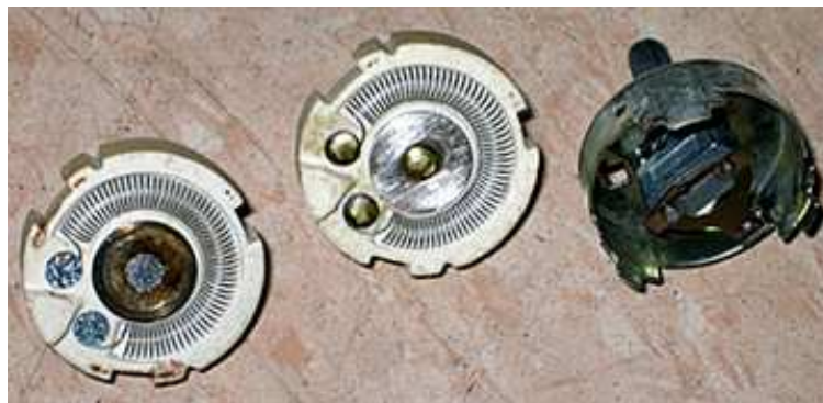
Fig. 3.13 Aetna-Pollak potentiometer before (Left) and after (Center/Right) restoration.
