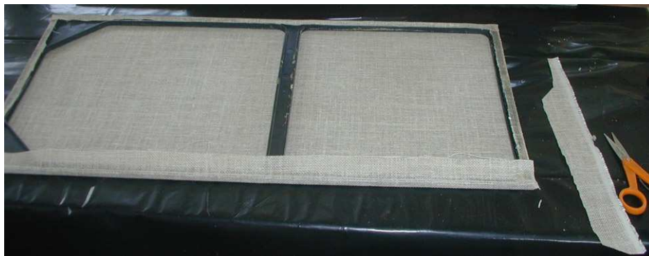
Fig. 3.20. Attaching grille cloth with gel contact cement.
