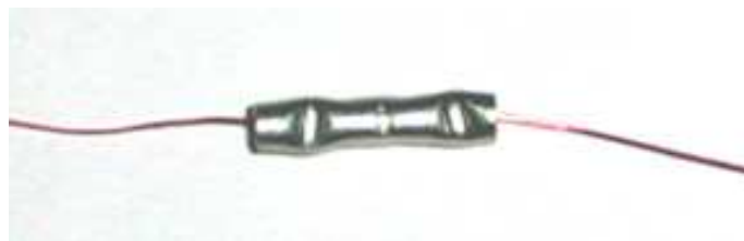
Fig. 4.3. Joining 0.0045-in.diameter wires with a crimp connector.
