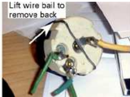
Fig. 3.11 Removing potentiometer bail
